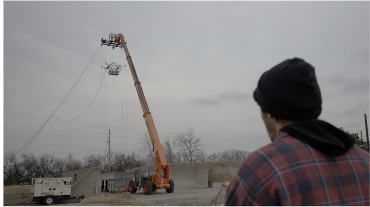
BETA partners with NIAR and FAA to conduct first-ever 50ft drop test of full-scale battery system
