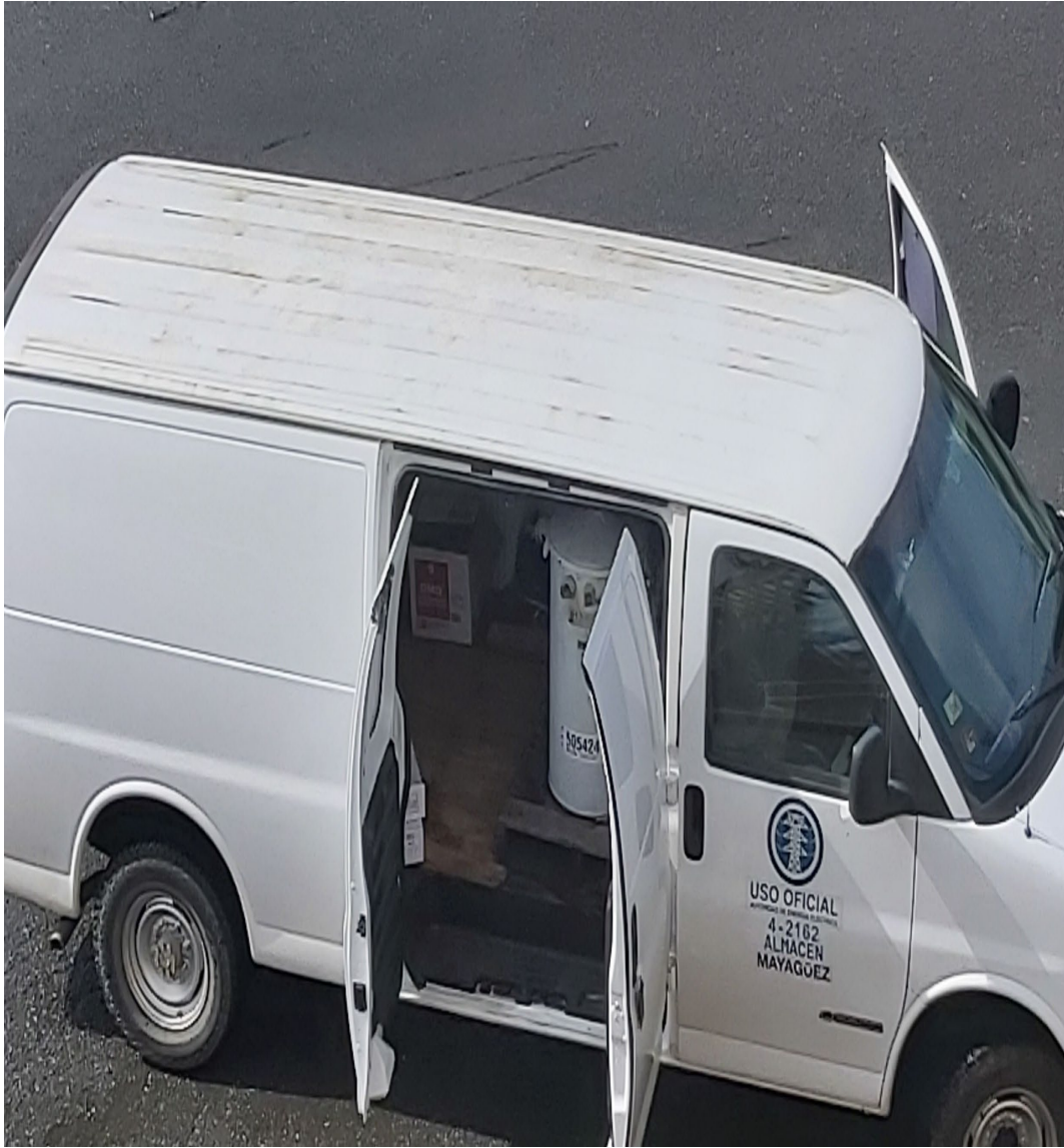
Palo Seco. Transformer transported in enclosed van, no spill tray, no tiedown.
