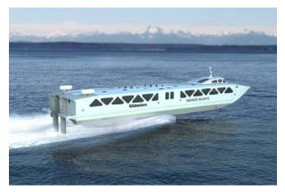
Glosten has partnered with Bieker Boats to form Foil Ferry, LLC. This new company's vision is to design and bring to market a modern, composite hydrofoil passenger ferry. This ferry requires less than half of the installed power of a typical, high-speed passenger catamaran and could utilize all-
