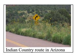
The above photo is typical in Indian country. A sign, listing the speed limit and warning of an upcoming curve, is obstructed by overgrown vegetation. Notice that the road has no
